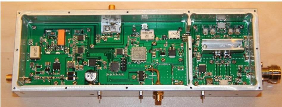
2: The bare module, but now included a milled and drilled waterproof housing. All the patch cables, connectors and a heatsink included. You can install the module yourself in the cabinet, cables on and ready.
